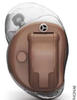
Illustration of an in-the-ear hearing aid
