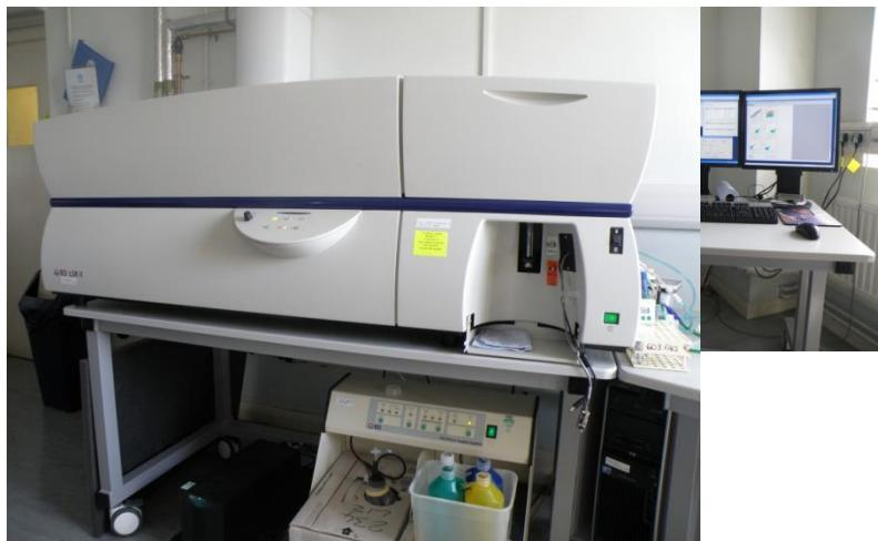
3 laser (B/R/V), 2 scatter, 14 fluorochrome (6/3/6) LSR-II flow cytometer for Multiparameter analysis.
